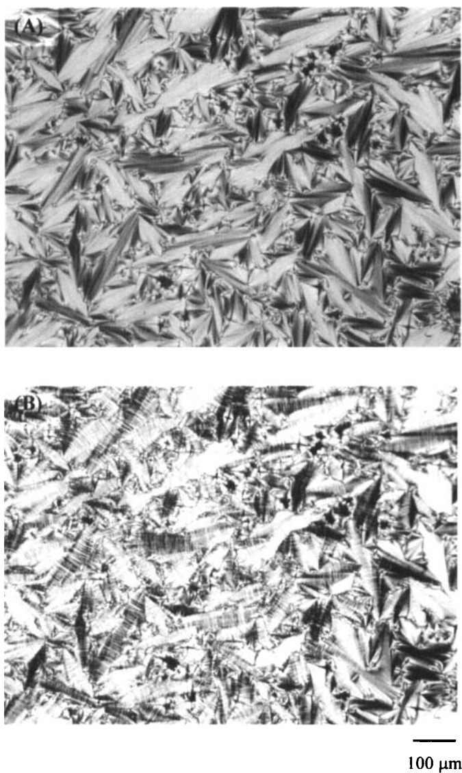
FIGURE 1 Polarizing optical micrographs of 1 at 170 °C (A) and at 144 °C (B). See Color Plate XXXI at the back of this issue.
